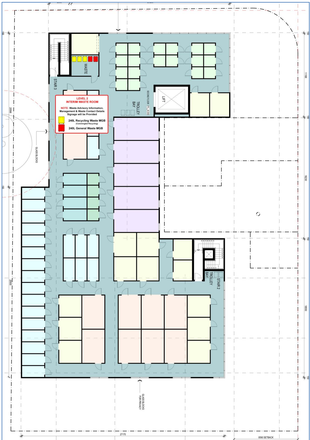
Figure 9: Scaled Diagram of Level 2 Waste Storage Room
